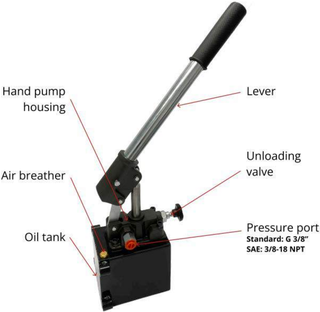
Photo 1. Main components of a single acting hand pump
